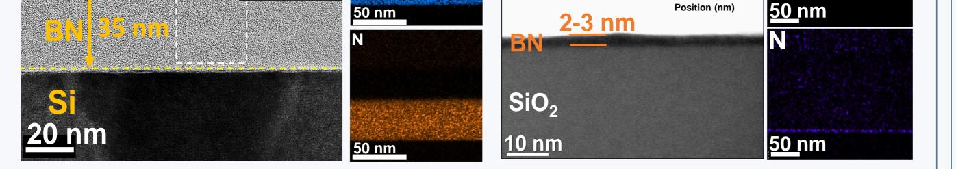
• Achieved a controllable uniform film thickness down to a few-nanometer thickness.
