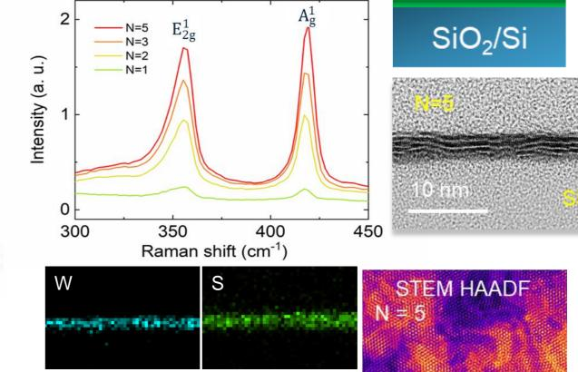
ALD WS<sub>2</sub> - layer by layer deposition at 350 °C
