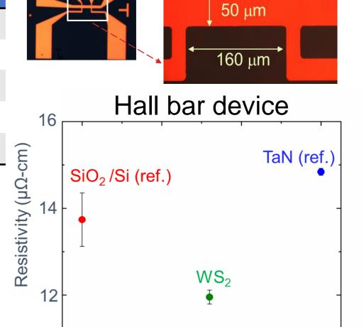
Liner thickness (nm) Cu film on WS<sub>2</sub> shows lower resistivity
