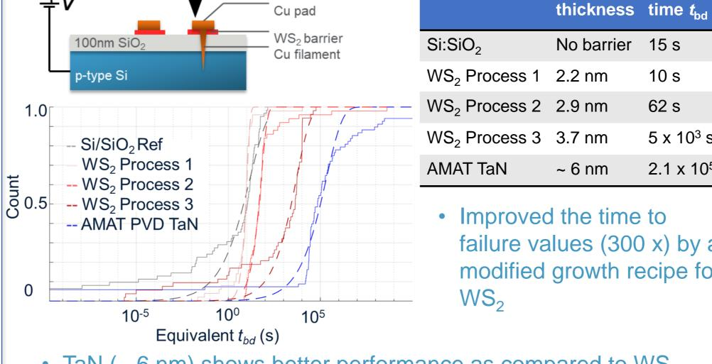
No barrier 15 s 2.2 nm 10 s WS<sub>2</sub> Process 2 2.9 nm 62 s WS<sub>2</sub> Process 3 3.7 nm  $2.1 \times 10^5 \text{ s}$ ~ 6 nm Improved the time to failure values (300 x) by a modified growth recipe for
