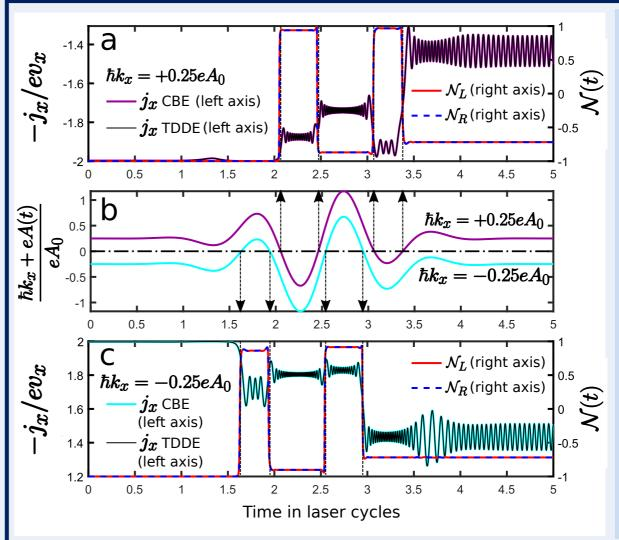
**Figure 1:** Time-evolution of (b) electron minimal-coupling momentum, and (a),(c) population difference (right axis) and single-electron current (left axis) for 2 starting momentum values. When the electrons are driven close to the Dirac point (horizontal dash-dotted line in (b)), instantaneous and complete population inversion occurs resulting in nonlinear current response.
